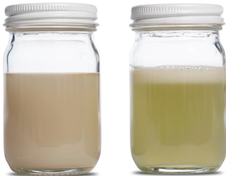
Bifender FC stays in suspension much longer than other fertilizer-compatible bifenthrin products. This photo was taken 6 hours after mixing with 10-34-0.
